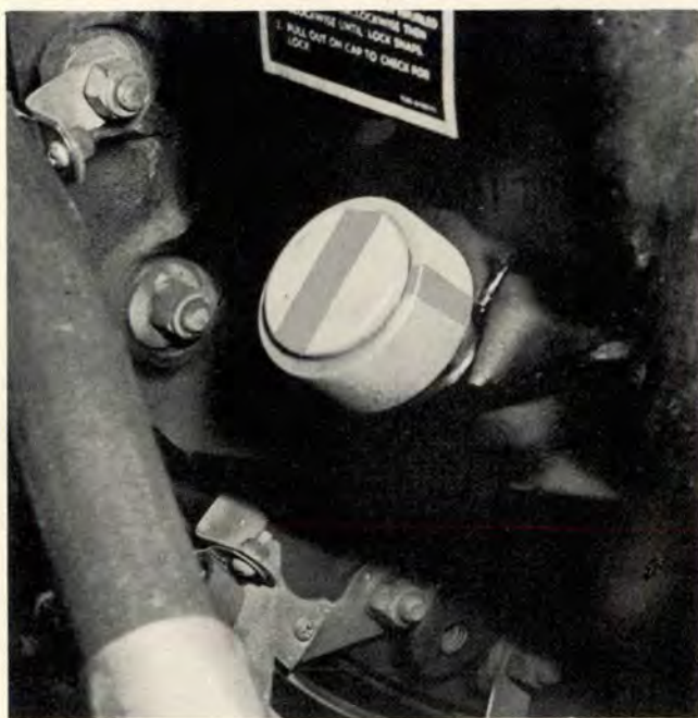
Left, the oil cap is down and in place on filler neck but not locked. Note the position of the painted aligning marks, indicating an unlocked condition. Right, painted aligning marks now indicate a locked condition, but oil cap is loose on filler neck. Cap must be fitted tightly, with markers aligned.
