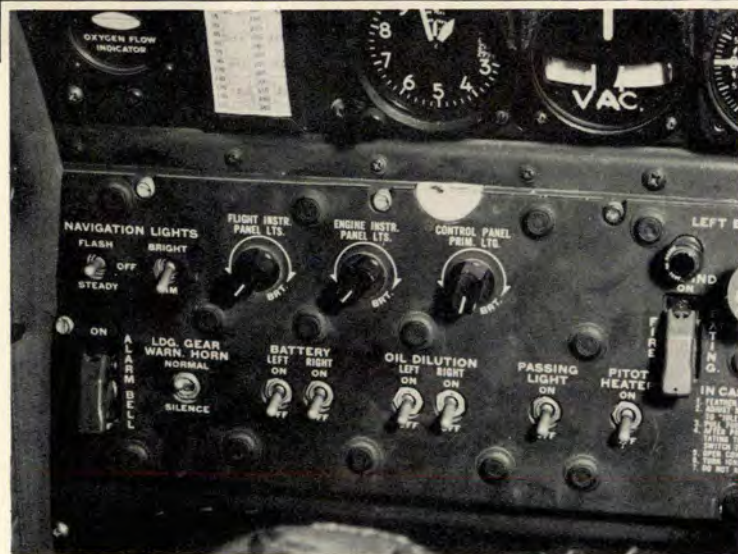
Above, the pilot's panel has been redesigned to present a logical arrangement of necessary switches. Left, engine fire extinguishers are relocated in nacelles.
