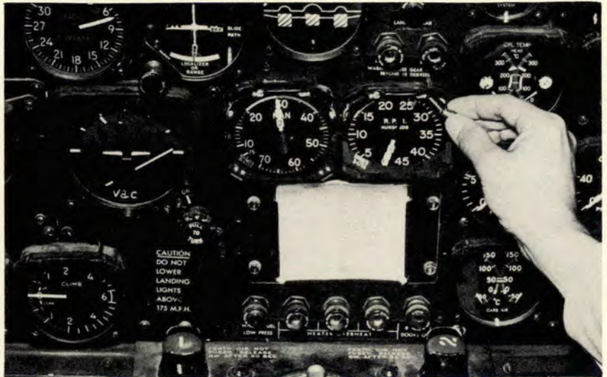
New cockpit lighting consists of red lights installed in small shields over every instrument on the panel. Shields pull down to facilitate easy bulb replacement from handy overhead box.
