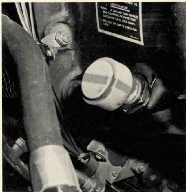
Left, the oil cap is down and in place on filler neck but not locked. Note the position of the painted aligning marks, indicating an unlocked condition. Right, painted aligning marks now indicate a locked condition, but oil cap is loose on filler neck. Cap must be fitted tightly, with markers aligned.
